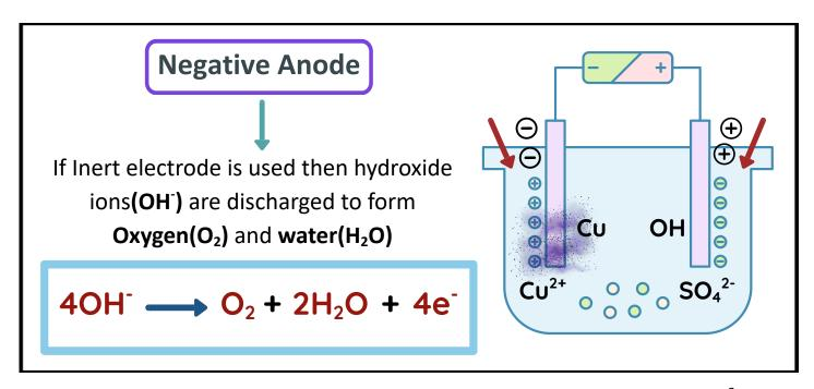
If the Anode is made of Copper it will dissolve in the solution as Cu<sup>2+</sup> while these ions in the solution deposit at Cathode.
