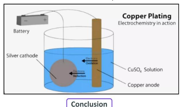
The Electrolysis of CuSO<sub>4</sub> involves transfer of Cu<sup>2+</sup> ions from solution to cathode, where they are reduced and deposited as copper metal. If Inert electrodes are used then Oxygen is produced at Anode. Sulphate ions remain in solution. If copper electrodes are used, the anode dissolves and form the copper ions in solution.
