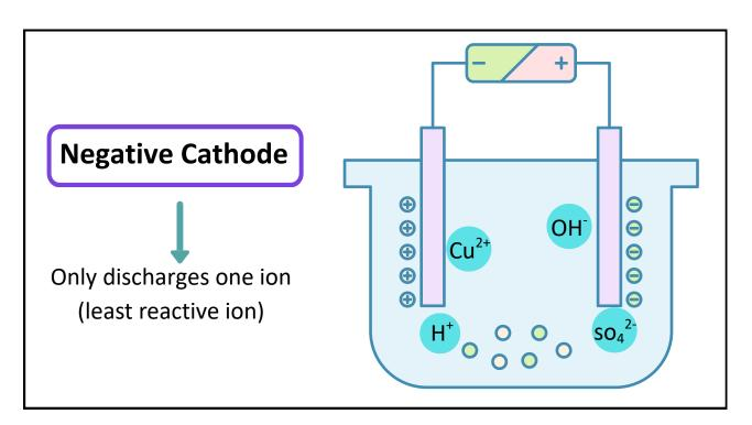
Copper ions gets discharged to form Copper metal which deposits at the cathode. Chemical Reaction -
